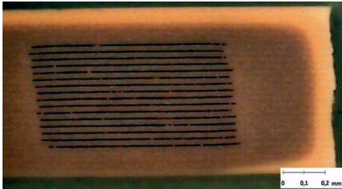
Figure 3.4.6: Cross section of MLCC of K85 + 5 wt% GL15 and Cu electrodes fired at 1040 °C in wet N 2 .
